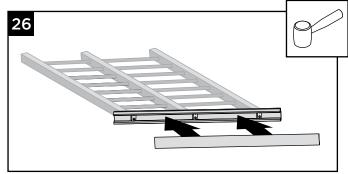
26. Using a mallet, install bottom rail cover onto bottom rail.
