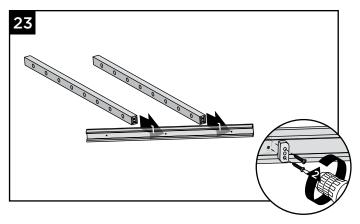
23. Install lowest end vertical and all intermediate verticals to bottom rail using ST Wedge Spacer and screws provided.
