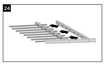
24. Slide rods into lower end and all intermediate verticals.
