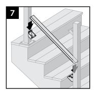
How to Mark, Cut and Place Top Stair Railing
