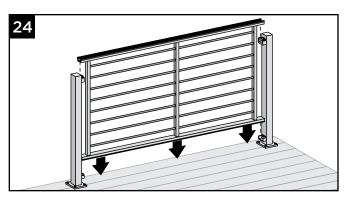
24. Drop assembled rod rail panel into brackets.
