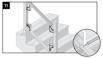
11. Using the long edge of the stair template, mark the location of the end verticals on the upper and lower rails.
