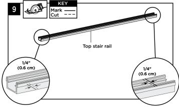
9. Cut each end of top stair rail and top rail cover 1/4" (0.6 cm) shorter than mark to allow for fit into top stair rail bracket.
