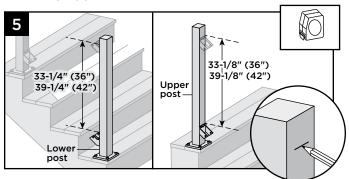
5. On Lower Post - From top of lower bracket, measure up and mark with light line (33-1/4" for 36" rail; 39-1/4" for 42" rail). On Upper Post - From top of lower (upper) bracket,
