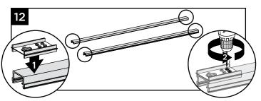
12. Place HZ template at end of top and bottom rails. Pre-drill pilot holes (using a 7/64" bit or small punch) at locations.
