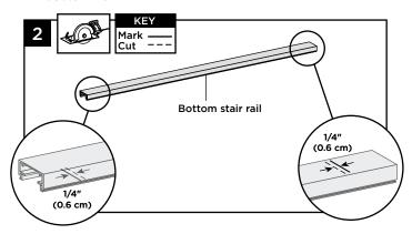
2. Cut each end of the bottom stair rail and bottom rail cover 1/4" (0.6 cm) shorter than the mark on each end to allow for fit into bottom stair rail brackets.
