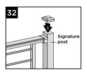
33. Attach post caps to post sleeves using external grade PVC construction adhesive.
