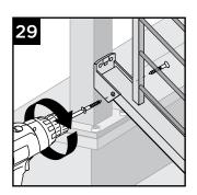
30. Attach top stair rail to top stair bracket (all types) using two self-tapping screws (provided) on each side of stair bracket.
