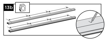
13b.Measure the distance between the vertical end holes on **both top and bottom rails**. Divide the distance into thirds and make two marks on top and bottom rails.
