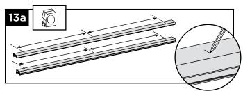
13a. Measure the distance between the vertical end holes on **both top and bottom rails**. Mark the center.
