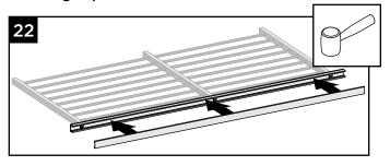
22. Using a mallet, install bottom rail cover onto bottom rail.
