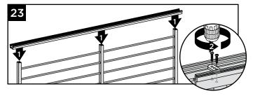
23. Install top rail to all vertical and end supports using HZ spacer and screws provided.
