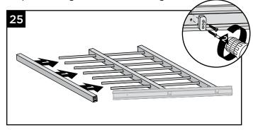
25. Slide upper end vertical onto rods and attach to bottom rail using ST Wedge Spacer and screws provided.
