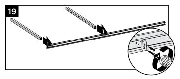
19. Attach **one** end vertical and **all** intermediate verticals to bottom rail using HZ spacer and screws provided.
