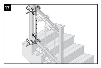
17. Clamp top vertical (upper part of stairs) in place, using width of stair template to position.
