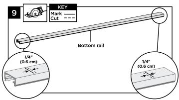
9. Cut each end of bottom and top rail 1/4" (0.6 cm) shorter than mark on each end to allow for fit into bottom rail brackets.
