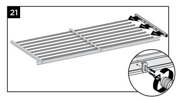
21. Slide end vertical onto rods and attach to bottom rail using HZ spacer and screws provided.
