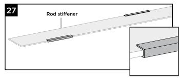
27. Attach tape (qty 6 provided) to alternating sides of the rod stiffener as shown.
