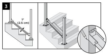
With deckboard still on nose of stair tread, place brackets on end of bottom stair rail (do not attach brackets to rail) and mark posts for bracket locations.
