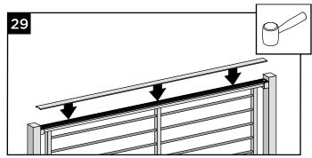
29. Using a mallet, install top rail cover.
