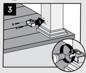
Measure up from decking surface 33-15/16" (862 cm) for 36" (92 cm) rail height or 39-15/16" (101.4 cm) for 42" (107 cm) rail height. Mark with light line.
