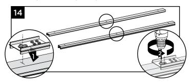
14. Using the slot on the HZ template, locate marked line and drill two 7/64" pilot holes (or mark with a punch).
