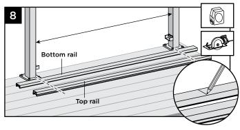
8. Position bottom and top rails between posts and align with bottom bracket. Mark bottom rail and top rail at each end.
