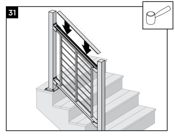
31. Using a mallet, install top rail cover.
